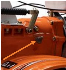
Fig. 5 – Checking the transmission oil level
